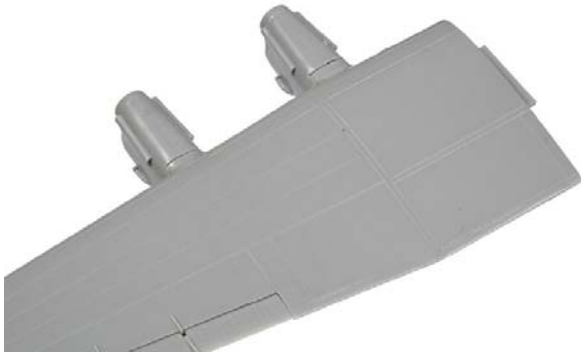
Above: The surface of the Airfix Lancaster is covered with tiny raised rivets. I decided to supplement these on the wings with recessed panel lines. These were marked out based on plans, and scribed using self-adhesive Dymo tape as a guide.
