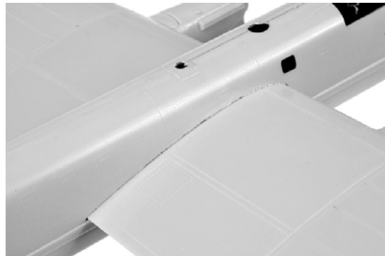
Above: Although the wings fitted snugly against the fuselage recesses at the wing roots, there were a few gaps that needed to be filled here
