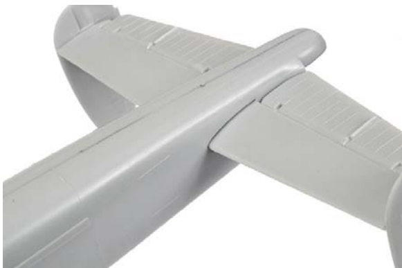
Above: The tailplanes sported a similar gap to the wing root
