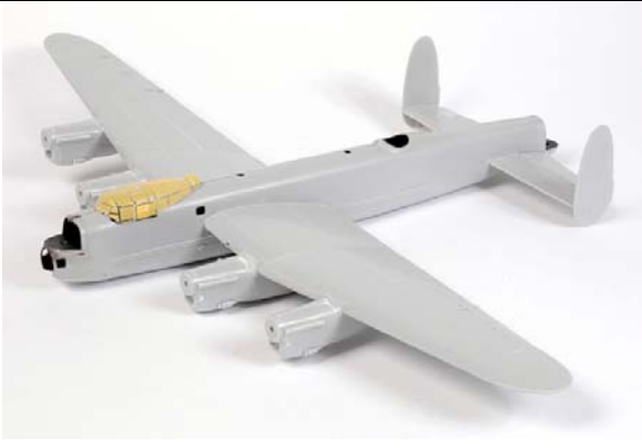
Above: Milliput, a white coloured two-part epoxy putty, was employed to fill the gaps at the wing roots, tail planes and the engine nacelles. Tamiya Surface Primer was applied over the top of the Milliput and sanded smooth when dry.
