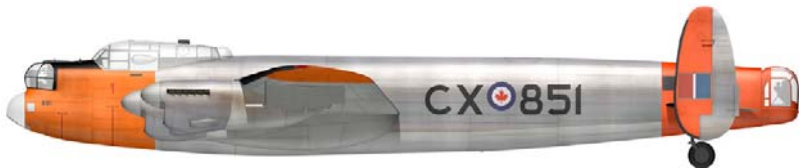
Lancaster Mk. 10DC. Used by the Canadian Air Force as a launch platform for 'Firebee' drones.
