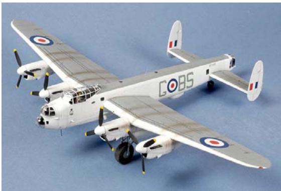
ABOVE: Weathering was generally kept fairly subtle, but the dark exhaust stains on top of the wings were frequently seen on the real aircraft. These stains were built up from fine streaks of heavily thinned paint.
