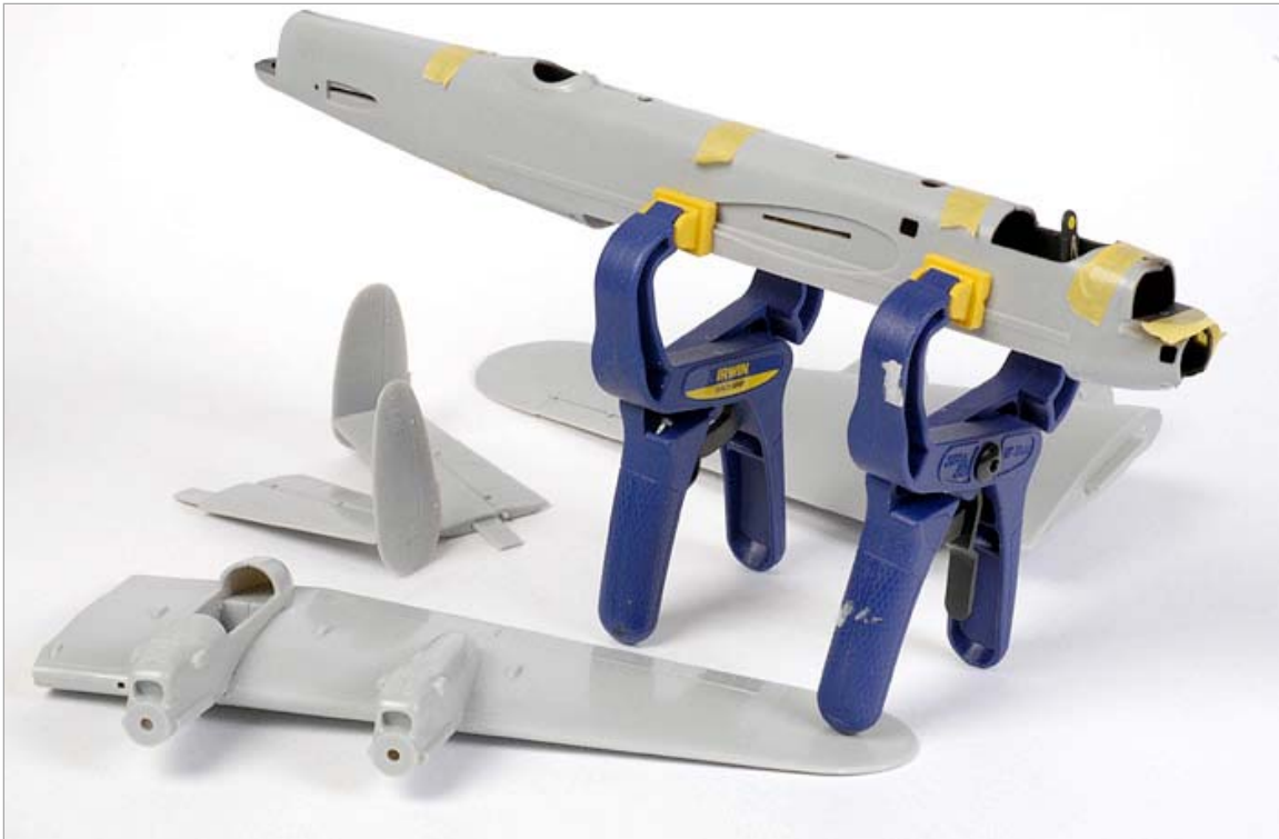
Above: The fuselage halves were clamped together to ensure accurate alignment.
