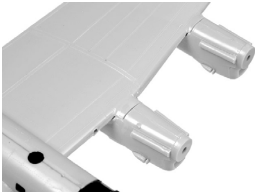
Above: The main areas that required additional attention were gaps between the engine nacelles and the leading edge of the wings
