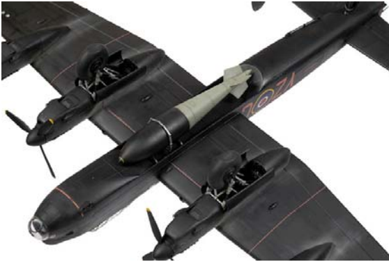
BELOW: The big Grand Slam bomb slung under the fuselage dramatically alters the profile of the Lancaster.
