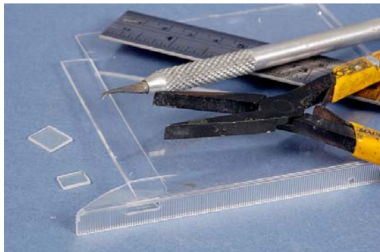
ABOVE: The Lancaster MR.3 was fitted with two additional windows in the rear fuselage. First, oversized rectangles were removed from the clear plastic using the "score and snap" method.
